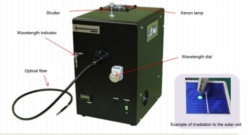
Generally, the irradiation light source configured with a xenon lamp and band pass filter is cheaper while it is not convenient since the irradiation wavelength cannot be selected without any restriction and different filters have to be prepared to use different wavelengths. The Model NIJI 2 Variable Wavelength Light Source is capable to perform irradiation at any wavelength in the range of 300~1150nm using the monochromator instead of the band pass filter.
